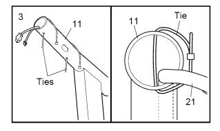
4. Place the Console Base (46) on the posts on the Upright. Make a loop with the indicated plastic ties and insert the two Wires (21) through the loops. Pull out only enough of the two Wires to connect them to the connectors in the Console Base. Plug the Wires fully into the connectors. Tighten the loops and cut off the excess plastic tie. WARNING: Do not disconnect or connect the Wires while the treadmill power cord is plugged in.
